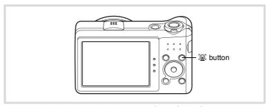
An icon indicating either Face Detection On or Smile Capture appears on the display. (The icon does not appear when the Face Detection function is not activated.)
